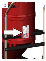
Connect to proper power source as indicated on the serial tag.
