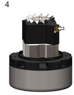
Carefully dislodge the plastic motor cap via the built-in hooks on both sides of motor brush. (TIP: Dislodge one side of a cap first followed by the other.)
