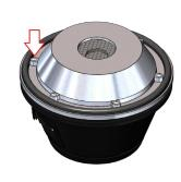
Remove the 6 screws attached to each motor assembly.
