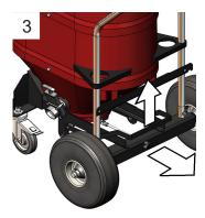
After the machine is completely drained, the bottom discharge may be used to remove excess sludge.
