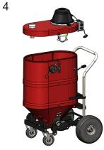
Remove motordeck and inspect foam filter. The filter is used to stop moisture from entering the motor and not for filtering dust.
