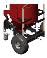
Check that the shutoff plate is forward, foot lever is locked, and slide valve is closed.
