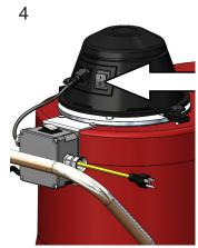
Start machine using the ON / OFF switch on the motor dome.
