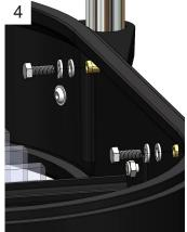
Insert M6 screws into the back of PEMs.
