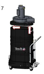
Replace the motor deck, attach the ground wire.
