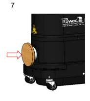
Place the vacuum under pressure by blocking the inlet and turning the machine on.
