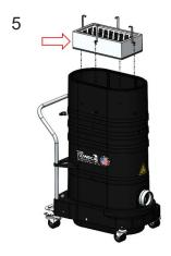
Remove and replace the HEPA filter.
