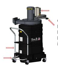
Check from continuity between the plug and handle bar, dustpan lever, and starter box if applicable.
