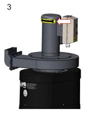
Turn motor on, then off quickly to confirm the motor is spinning in the correct direction.
