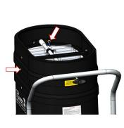
Insert the filter spacer hardware and reattach the ground wire.
