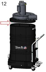
Replace the moto deck and connect the ground.
