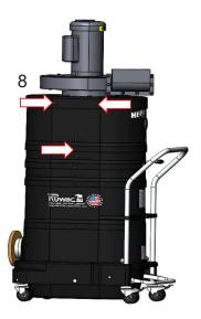
Drill holes into the housing with an 5/16in bit at the 6 locations pointed out above.
