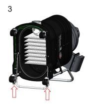
Lock the rear casters and carefully tip the machine back until it rests on the handle bar
