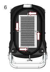
Tighten the bracket hardware.
