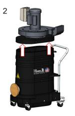
Remove the motor deck.
