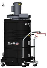
Use the filter shaker to clean the filter before and after each use.
