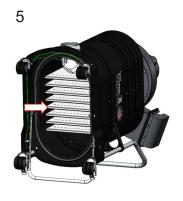
Inspect filter pleats for any tears or damage. Inspect the inlet deflector for wear as well
