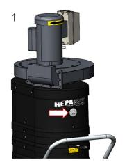
To ensure optimal performance of the HEPA Maxx filter, replace when the head loss reaches 8 inches of water column.
