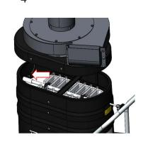
Turn vacuum on and block the inlet to place vacuum under pressure.
