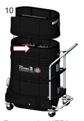
Remove the HEPA module. Drill holes with a 1/2in bit at the 2 locations point out above.
