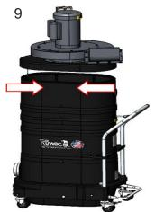
Remove the motor deck. Drill holes with a 1/2in bit at the 4 locations pointed out above.
