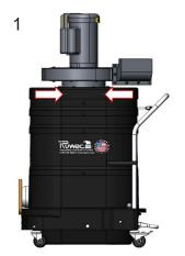
Remove the motor deck hardware.
