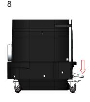
Push the lever down to secure the dustpan
