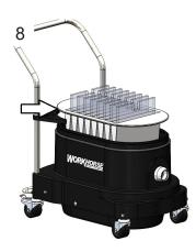
Remove and replace the filter. Keep the black mesh inserts.
