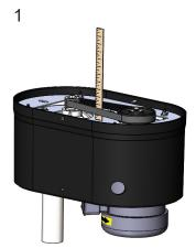
Measure the height of the first groove on the turbine sheave. Check that the first groove of the motor sheave matches this height.
