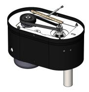
Re-install the belt and adjust to proper tension (see pg. 13).
