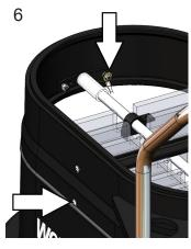
Disconnect the filter ground and remove the filter spacer hardware.
