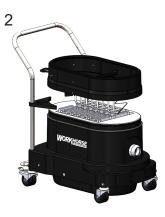
Insert the filter cage into the filter pleats.
