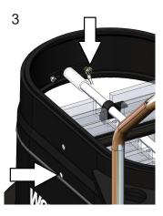
Insert the filter spacer hardware and reattach the ground wire.
