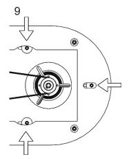
Replace turbine by fastening all nuts and bolts through bottom of motor deck.
