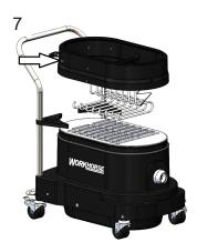
Remove the filter ring and shaker assembly.
