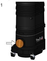
Turn vacuum on and block the inlet to place vacuum under pressure.
