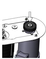
Once motor sheave is at correct height, tighten bolt to 15 ft-lbs of torque.
