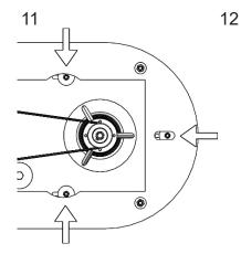
Tighten all nuts and bolts surrounding turbine to ensure they're resting front end on a fastened snug securely. Do not overtighten.
