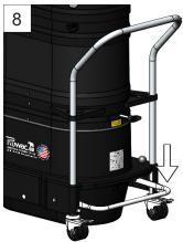
Push the lever down to secure the dustpan
