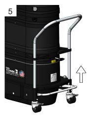
To empty the machine, release the dustpan lever.
