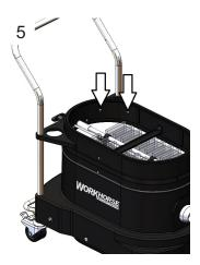
Remove the handle bar bracket hardware.
