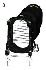
Lock the rear casters and carefully tip the machine back until it rests on the handle bar
