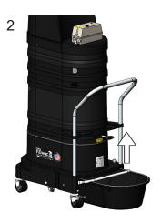
Pull up the lever and remove the dustpan
