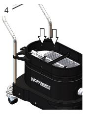
Install the handle bar bracket hardware.
