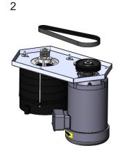
If motor sheave needs adjustment, remove belt and adjust motor sheave (see pg. 10 for belt removal instructions).
