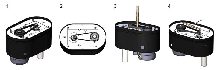
With power disconnected, remove the motor deck. Place the motor deck upside-down on a clean working surface.
