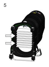
Inspect filter pleats for any tears or damage. Inspect the inlet deflector for wear as well
