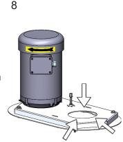
Using a sharp edge, remove the remaining silicone seal from the motor deck.
