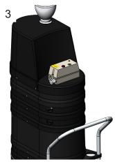
Quickly turn motor on/off to confirm it is spinning CW. Phase Indicator light on the starter should be OFF if spinning CW. If light is on switch red/black at cord cap. Power leads must be switched by licensed electrician.
