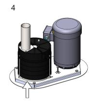
Break the silicone seal surrounding turbine using a sharp edge.
