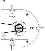
Loosen the three nuts securing the turbine, supporting it from underneath to ensure it doesn't drop.
