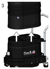
Remove the motor deck and silencer.
