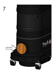
Place the vacuum under pressure by blocking the inlet and turning the machine on.
