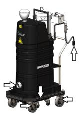
Also check for continuity between the plug and inlet, all four casters, and frame hardware if applicable.
