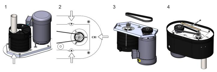
To replace a drive belt, first cut and remove silicone around turbine.
