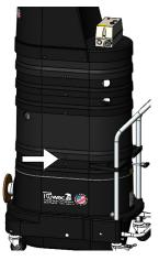
Remove all motor deck screws while the vacuum is under pressure. Turn off the vacuum after screws are removed.
