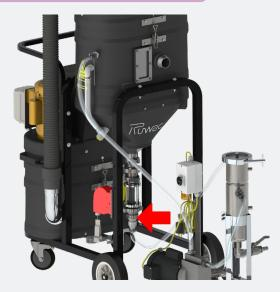
A. Connect the MXR to the discharge port of the MX360 unit.
