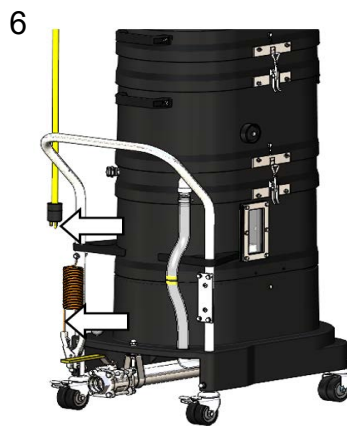
6 Power cord line ground to grounding cable hand clamp.
