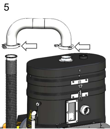
5 Release the sanitary clamp of the connection hose and elbow and remove the sanitary elbow.
