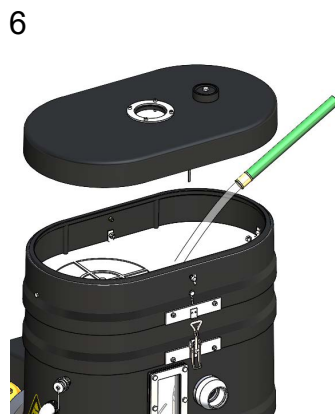
6 Remove the lid by unscrewing its hardware. Backwash the demisting pad by rinsing thoroughly with water.
