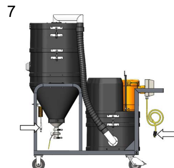
7 Power cord line ground to grounding cable hand clamp.
