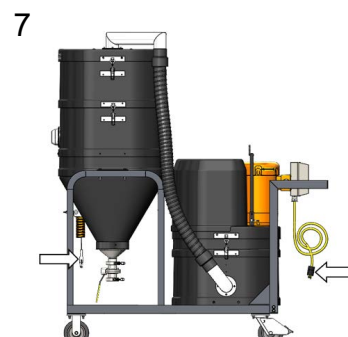
Power cord line ground to grounding cable hand clamp.
