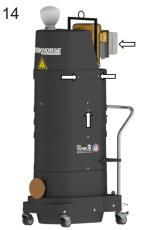
Insert <sup>1</sup>/<sub>4</sub>-20 bolts with lock washers into the 6 locations pointed out above.
