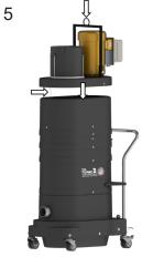
Place the motor deck on top of the HEPA module and connect the ground wire.
