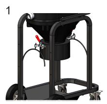
Move handles into the up position to open the bag clamps.
