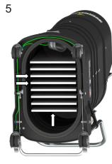
Inspect filter pleats for any tears or damage. Inspect the inlet deflector for wear as well
