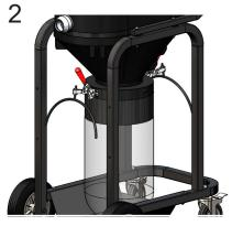
Open the bag completely and wrap it around the direct bagger barrel.
