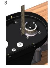
Loosen motor sheave hardware, and slide up or down as necessary.
