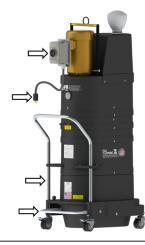
Check continuity between the cord ground line and handle bar, dustpan lever, and starter box if applicable.
