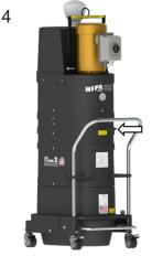
Use the filter shaker to clean the filter before and after each use.
