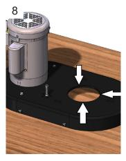
Using a sharp edge, remove the remaining silicone seal from the motor deck.
