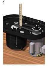
Measure the height of the first groove on the turbine sheave. Check that the first groove of the motor sheave matches this height.
