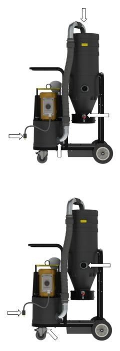
Check continuity between the cord ground line and elbows and continuous bagger hardware
