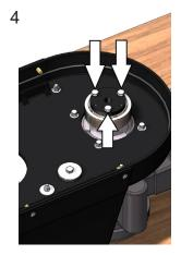
Once motor sheave is at correct height, tighten bolts to 15 ft-lbs of torque.
