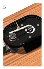
Re-install the belt and adjust to proper tension. (See pg. 18)
