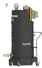
Place the vacuum under pressure by blocking the inlet and turning the machine on.
