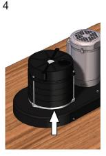
Break the silicone seal surrounding turbine using a sharp edge.
