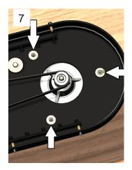
Loosen the three nuts securing the turbine, supporting it from underneath to ensure it doesn't drop.
