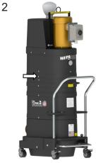
Remove all motor deck screws/HEPA MAXX screws if applicable; while the vacuum is under pressure. Turn off the vacuum after screws are removed
