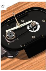
Check tension using a straight edge and tension gauge as shown above. (See pg. 18 for belt tensioning instructions)
