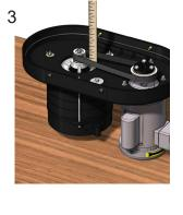
Check that sheaves are properly aligned. (See pg. 19 for pulley allignment instructions)
