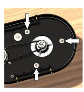
Loosen the turbine hardware, then slide turbine towards the motor to loosen the belt.
