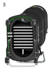
Lock the rear casters and carefully tip the machine back until it rests on the handle bar
