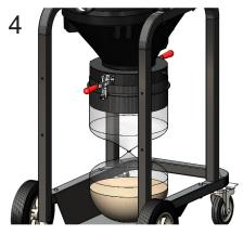
When removing material, tie off the bag before opening the bag clamps. Keep vacuum on while changing bags to ensure valve stays shut.
