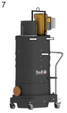
Drill/transfer holes into the housing with an 5/16in bit at the 6 locations pointed out above.
