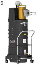
Turn on the motor before removing the dustpan. This will ensure that excess material sticks to the filter.
