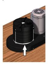
Once the belt has been properly tensioned. secure the hardware and re-seal the turbine with silicone.
