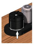
To replace a drive belt, first cut and remove silicone around turbine.
