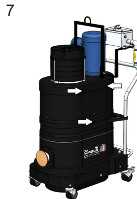
7 Drill holes into the housing with an 5/16in bit at the 6 locations pointed out above.
