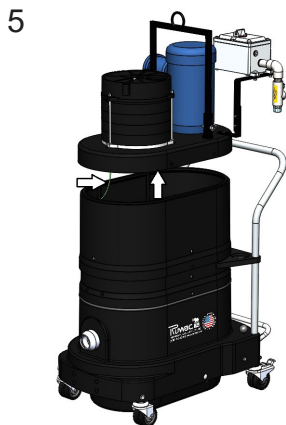
5 Place the motor deck on top of the HEPA module and connect the ground wire.
